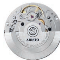
Sellita SW 200-1 Automatic-Werk Caliber 11 1/2, 26 Steine 28.800 A/h, Sekunden-Stopp
